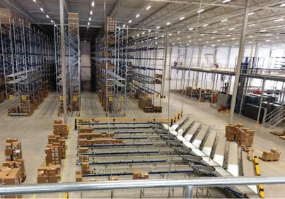
Technology: double-sided pop-up sorting, where cartons are dynamically lined out to the correct side right before sorting.
