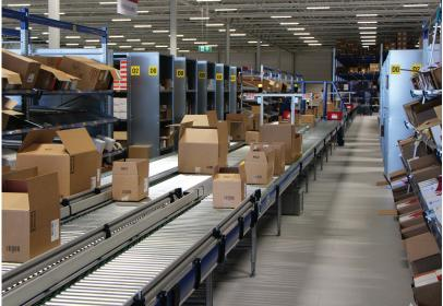
Cartons are transported to one of the 16 'zone picking workstations', where they receive the needed articles and follow their path to the next workstation or towards the packing process.
